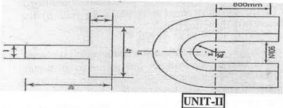
Design a journal bearing for a centrifugal pump with the following data. CO2 3 12M Diameter of journal =150mm Load on bearing =40kN
